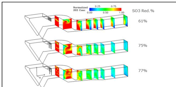
CFD predictions of SO<sub>3</sub> concentration and reduction percentage for a DSI system on a 450-MWe unit for 3 Cases with injection lances.
