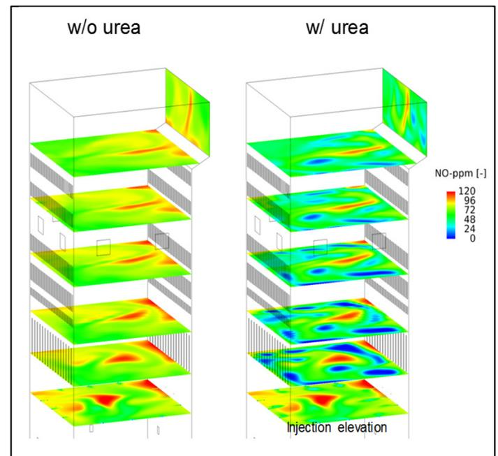
Model of furnace outlet NO<sub>x</sub> concentration without (left) and with urea injection (right) for a 350-MWe tower furnace burning lignite.
