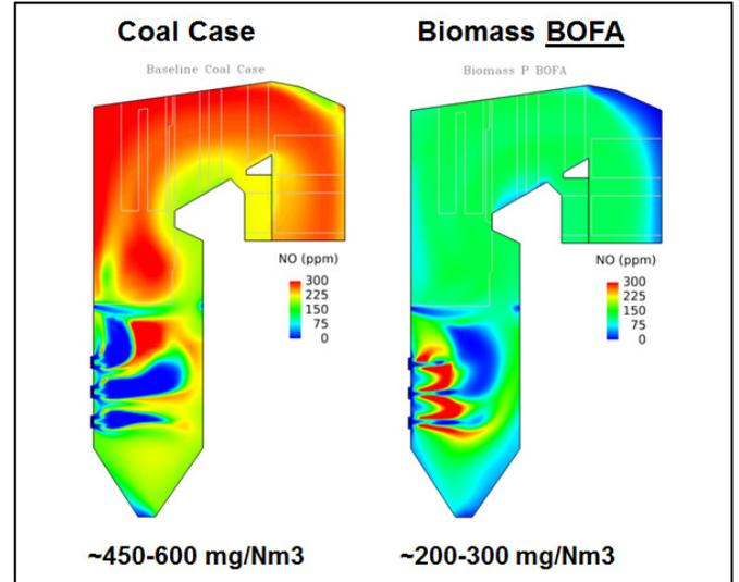
*CFD modeling of coal-to-wood conversion for a 500 MW wall-fired furnace. Modeling shows predicted NOx emissions between coal and biomass with BOFA NOx reduction technology.*
