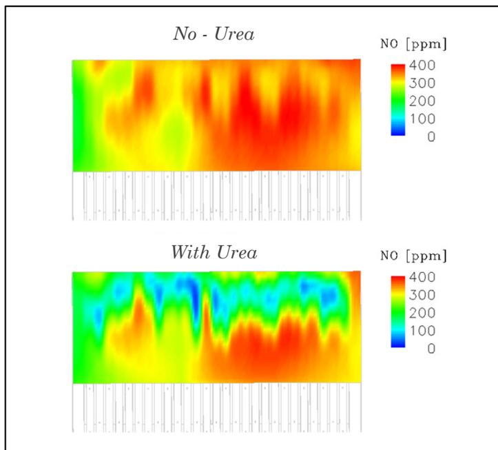
Model of furnace outlet NO<sub>x</sub> concentration without urea injection (upper) and with urea injection (lower) for a 420-MWe wall-fired unit.
