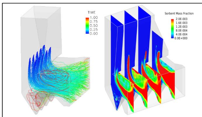
CFD model to determine injection locations and number of injections to obtain the best coverage of sorbent downstream before airheater inlet
