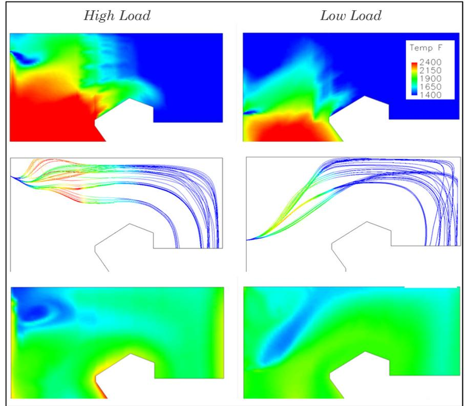
Models of furnace temperature (upper), urea injection trajectory (middle) and NO<sub>x</sub> concentration (lower) of SNCR system, as applied to a 700 MW boiler.
