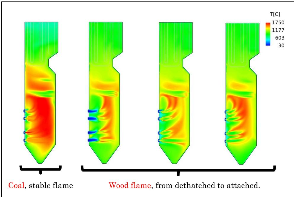
*CFD modeling of coal-to-wood conversion for a 500 MW wall-fired furnace. Modeling shows significant combustion differences between fuels and burner settings*
