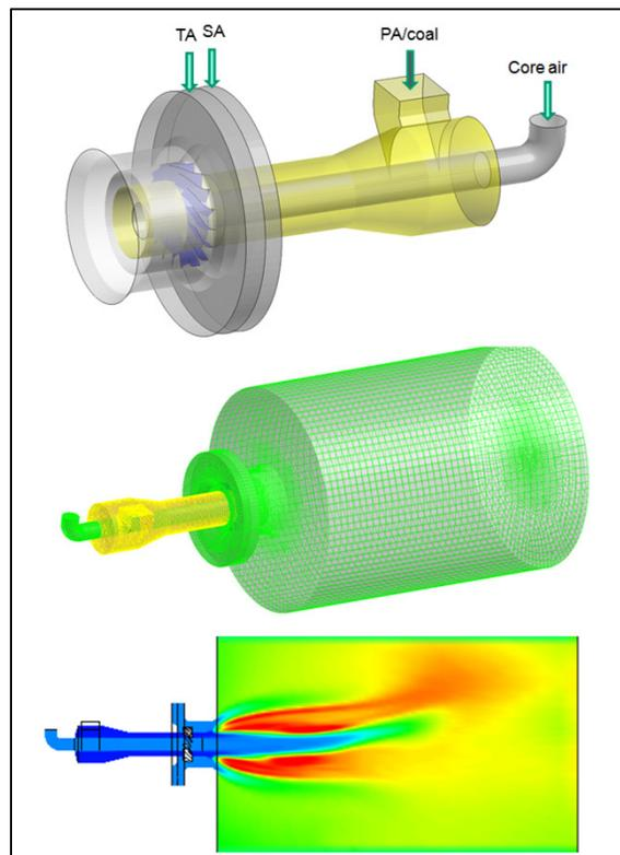
Model of single burner combustion
