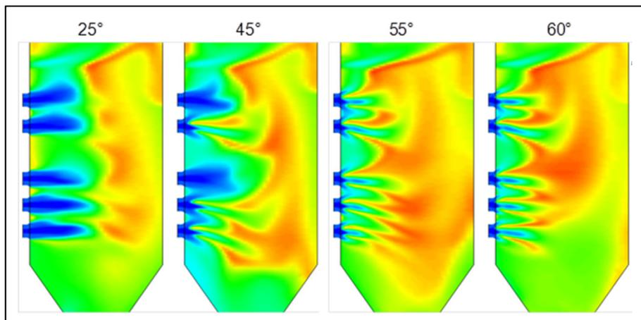
CFD modeling shows the change of flame shape when secondary air swirling angle increases from 25° to 60°
