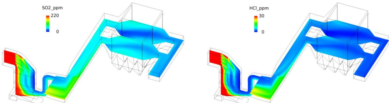
Fig. 2. CFD predictions of (left)  $\text{SO}_2$  and (right) HCl species concentration a DSI hydrated lime injection on a 200-MWe unit.
